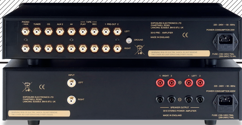
ABOVE: The 3510 pre [top] offers five line inputs (one for an MM/MC phono option), a tape loop and two preamp outs on RCA. The 3510 power amp [bottom] includes RCA inputs and dual 4mm speaker cable sockets (for bi-wire applications) but are for banana plugs only, so there is no provision for bare wire or spades here
