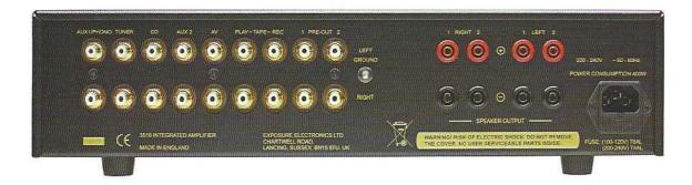
Plenty of connectivity here, with no fewer than six line inputs - the first of which can be fed by an internally fitted DAC or phono stage option. The gold-plated chassis-mounted phono sockets, together with the two sets of parallel-connected 4mm speaker sockets, are hand-wired.
