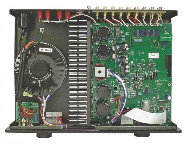
Excellent internal construction – as shown here. Of note: encapsulated relays for source switching (top right) and motorised Alps volume control (bottom right). Two pairs of output devices, mounted on a mid-section heatsink, are used for each power-amplifier channel. Powering it all is a hefty toroidal mains transformer (left).
