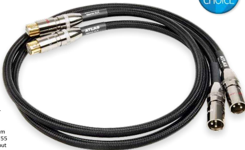
Silver betters both copper and gold for electrical conductivity, as reflected in the Mavros's 70mohm/m loop resistance, slightly higher than the Asimi's 56mohm. Otherwise, the Mavros Ultra offers a lower capacitance and, usefully, lower inductance at 82pF/m (86pF, Asimi) and 0.25µH/m (0.45µH), respectively. So the Mavros Ultra remains a fine choice for long runs.
