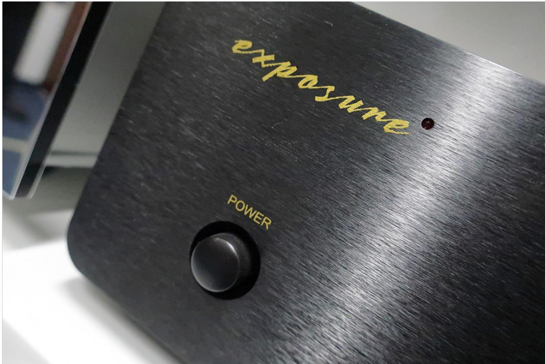
Manufacturer specifies frequency range 1 - 57 000 Hz (-3 dB), total harmonic distortion below 0.005% (1.6 V RMS / 1 kHz), signal and noise ratio 98 dB (1.6 V RMS / 1 kHz) and separation channels over 60 dB (20 - 20 000 Hz, at 1 kHz over 85 dB).
