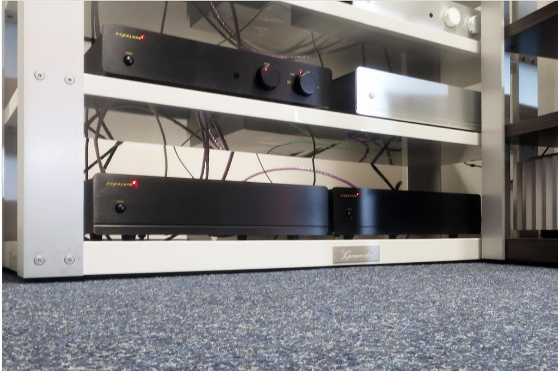
Each monoblock offers a bold output power of 200 watts to 8 ohms and 370 watts to half load, respectively. The amplifier operates in the frequency range 1 - 52 000 Hz (-3 dB), total harmonic distortion at full power up to 8 ohm does not exceed 0.015%, signal and noise ratio is very solid 120 dB or more (again at 200 W / 8 ohm).
