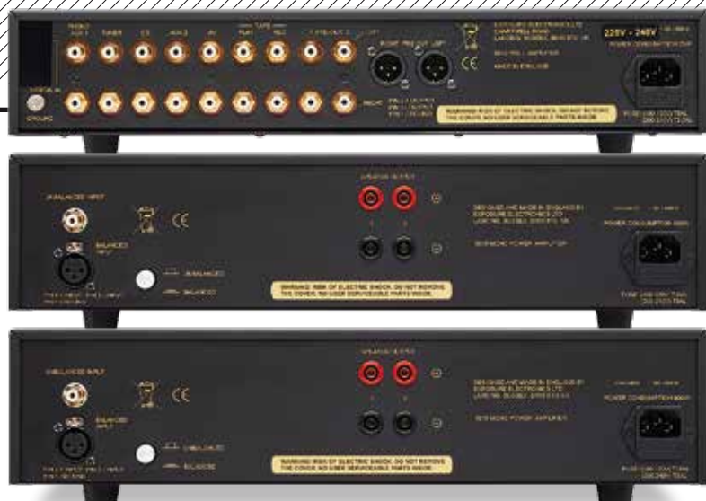
ABOVE: The preamp [top] offers five line inputs (one for an MM/MC phono option), a slot for a digital/DAC option, a tape loop and three preamp outs (two on RCA and one balanced on XLR). The power amp [below] has dual 4mm sockets that support bi-wiring. The input is single-ended (RCA) or balanced (XLR)
